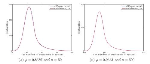
FIG 3: The stationary distribution of the customer number in the  $M/H_2/n$  queue, computed (i) by the finite element algorithm for the diffusion model with the reference density in (3.21) and (3.22), and (ii) by the matrix-analytic method.
