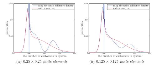
FIG 7: The stationary distribution of the customer number in the  $M/H_2/n + M$  queue, with  $\rho = 1.045$  and n = 500, computed (i) by the finite element algorithm using the "naive" reference density and different meshes, and (ii) by the matrix-analytic method.
