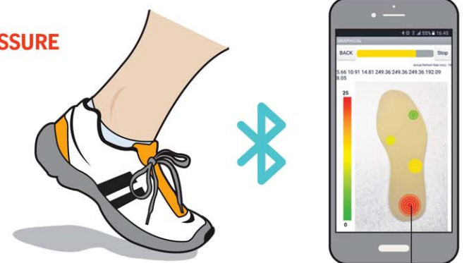
Mobile app: Pressure points are colour-coded to show the amount of stress on each point
