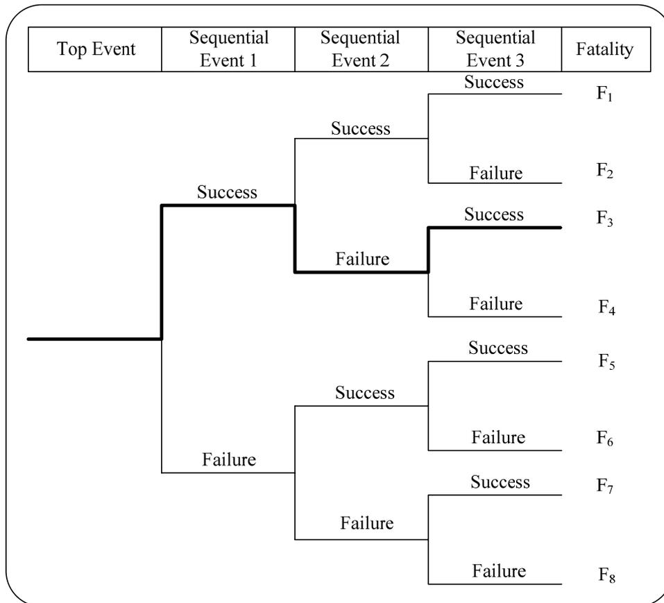
Figure 3 Example of Branch-based generic consequence estimation method
