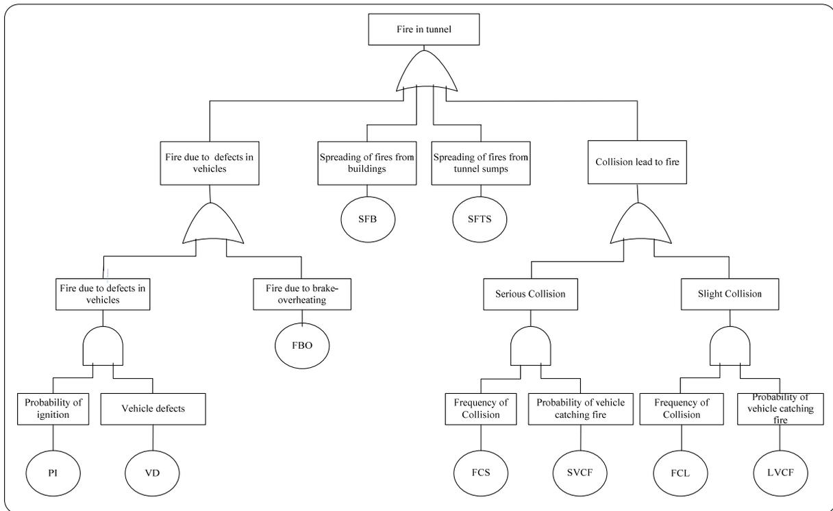
**Figure 1** Fault tree for fire in tunnel top event
