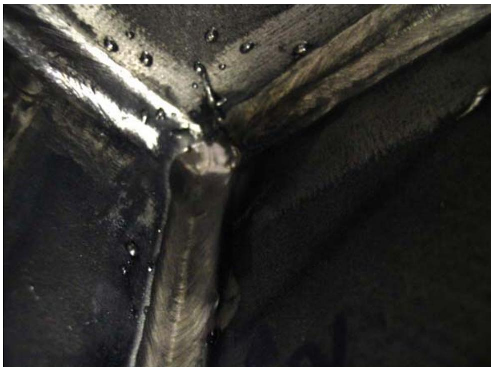
*Figure 13.* Production of spatter in overhead corner area of overlapping fillet welds.
