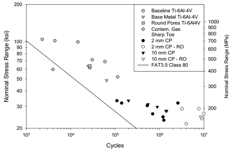
Figure 6. Fatigue performance of butt welds in tension.
