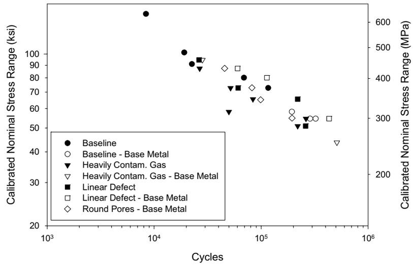
Figure 3. Fatigue performance of butt welds in four-point bending.
