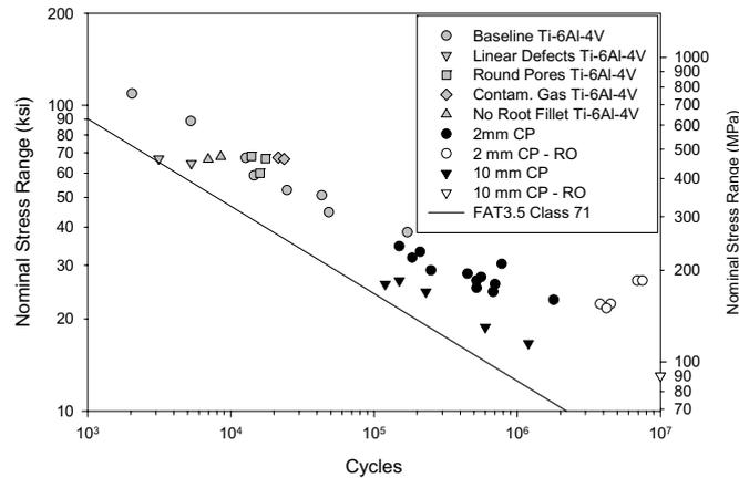
Figure 8. Fatigue performance of tang and slot welds in tension.
