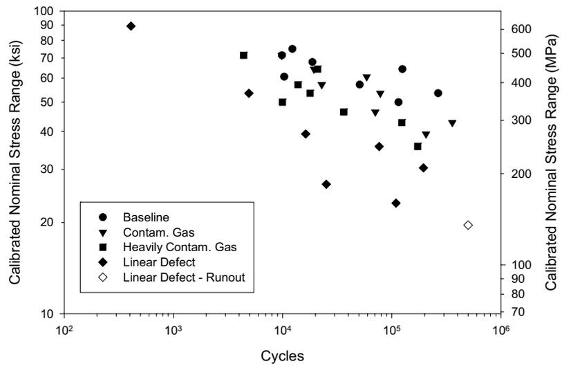
Figure 4. Fatigue performance of corner joints in 4-point bending.
