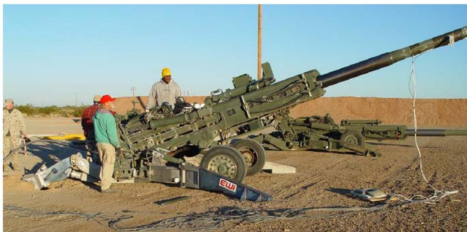
Figure 10. M777 155-mm howitzer with many titanium components.
