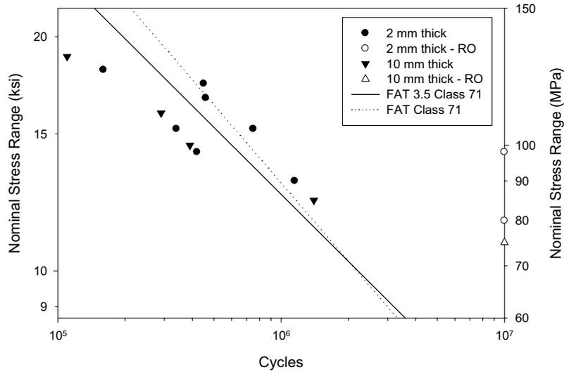
Figure 9. Fatigue performance of longitudinal attachment ends in CP Ti.
