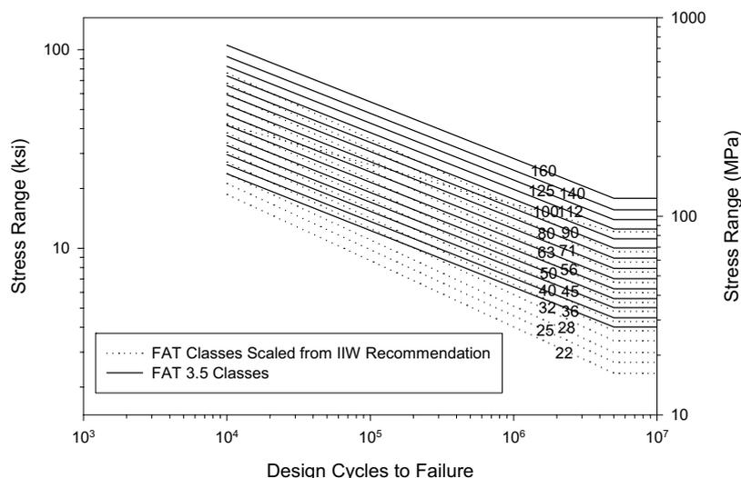
Figure 1. FAT and FAT3.5 class fatigue design curves.
