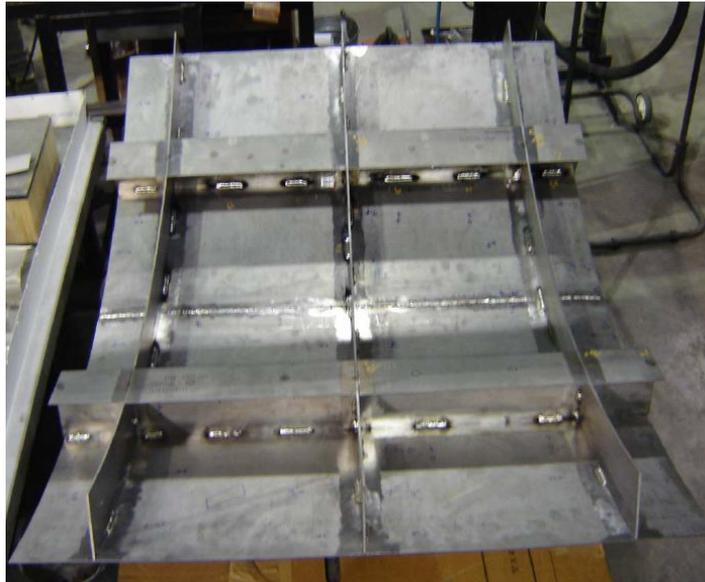
Figure 11. Mock-up structure in thin section titanium.
