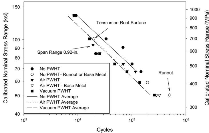
Figure 2. Fatigue performance of butt welds with differing PWHT in bending.
