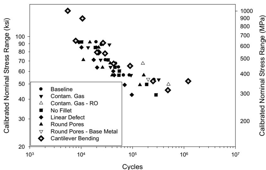
Figure 5. Fatigue performance of tang and slot model welds in bending.
