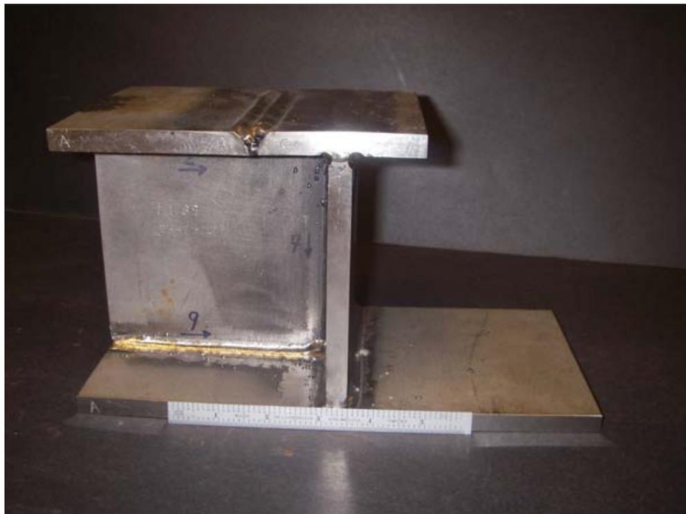
*Figure 12.* Mock-up of sliding door section.
