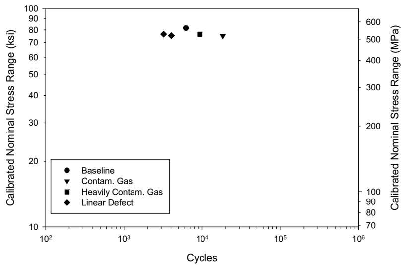
Figure 7. Fatigue performance of corner joints in remote tension.
