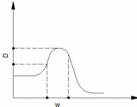
Figure 6. Determination of  $\tilde{d}_n$  corresponding to a  $\tilde{\omega}_n$  for a generic response spectrum
