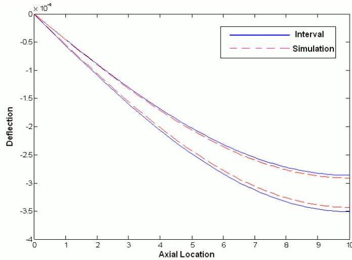
Figure 9. Beam deflection for the first three-mode response for example problem
