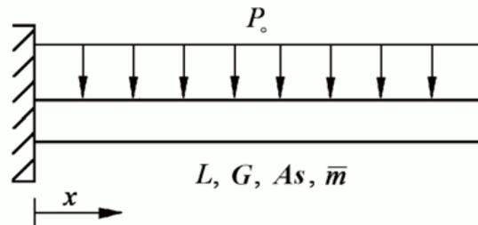
Figure 3. Cantilever shear beam with uniform dynamic load
