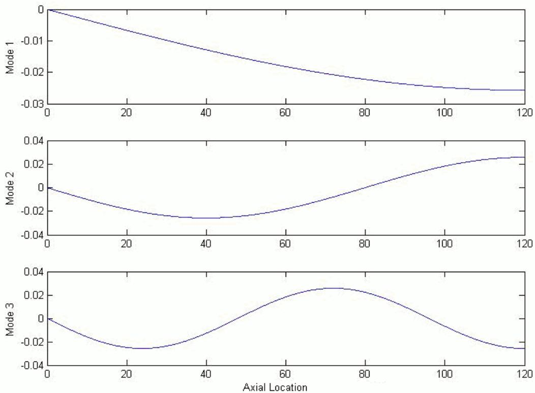
Figure 8. Beam deflection for the first three-mode response for example problem
