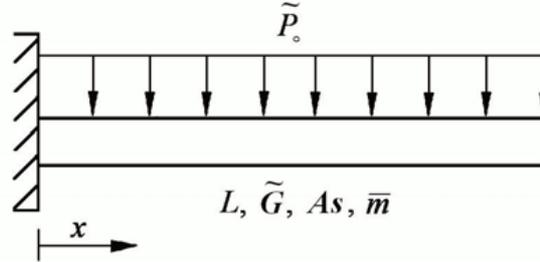
Figure 7. Cantilever shear beam with uncertainty in shear modulus and magnitude of uniform dynamic load
