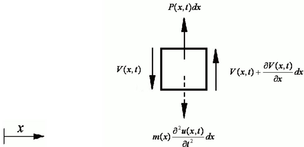
Figure 2. An infinitesimal segment of the shear beam
