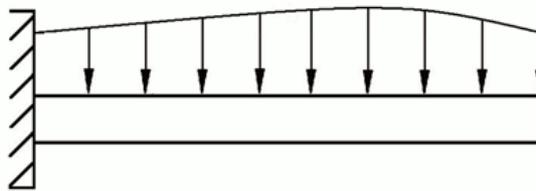
Figure 1. A general shear beam
