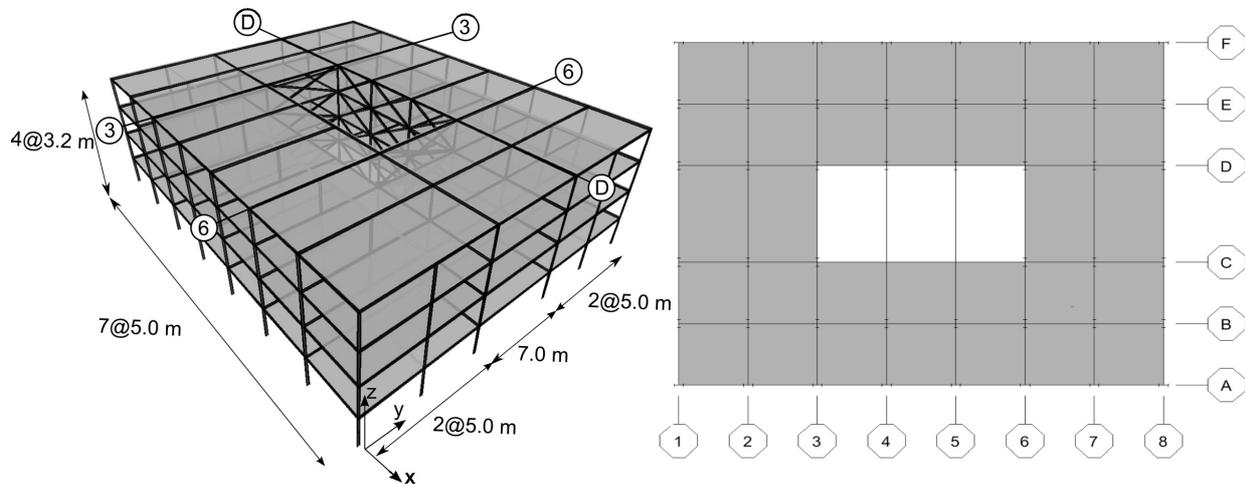
Figure 1. Isometric and plan view of the finite element model
