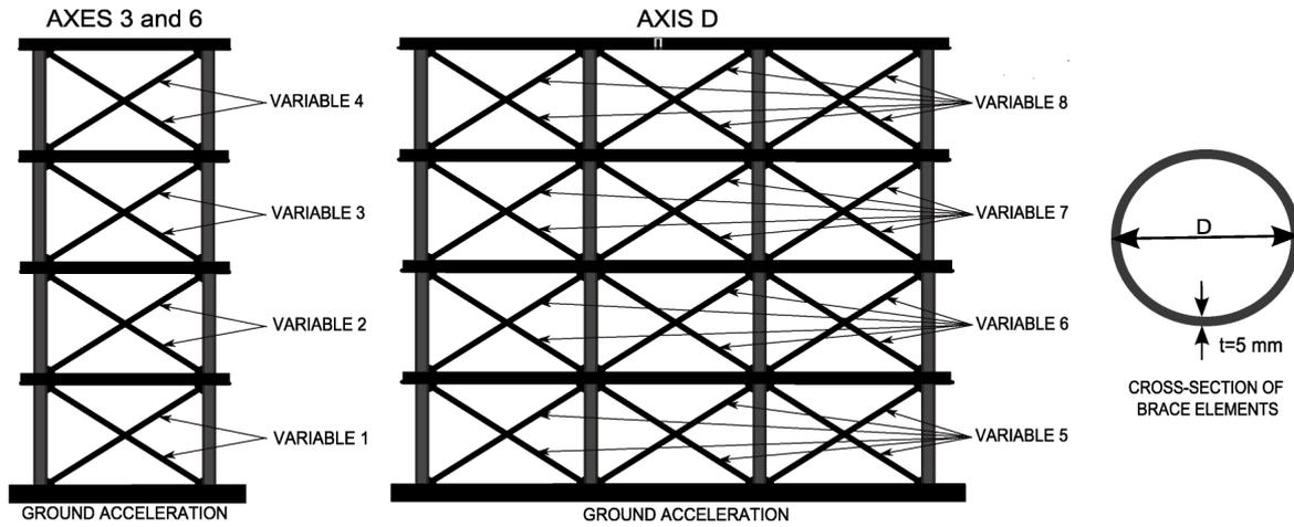
Figure 2. Axes 3, 6 and D of the structural model.
