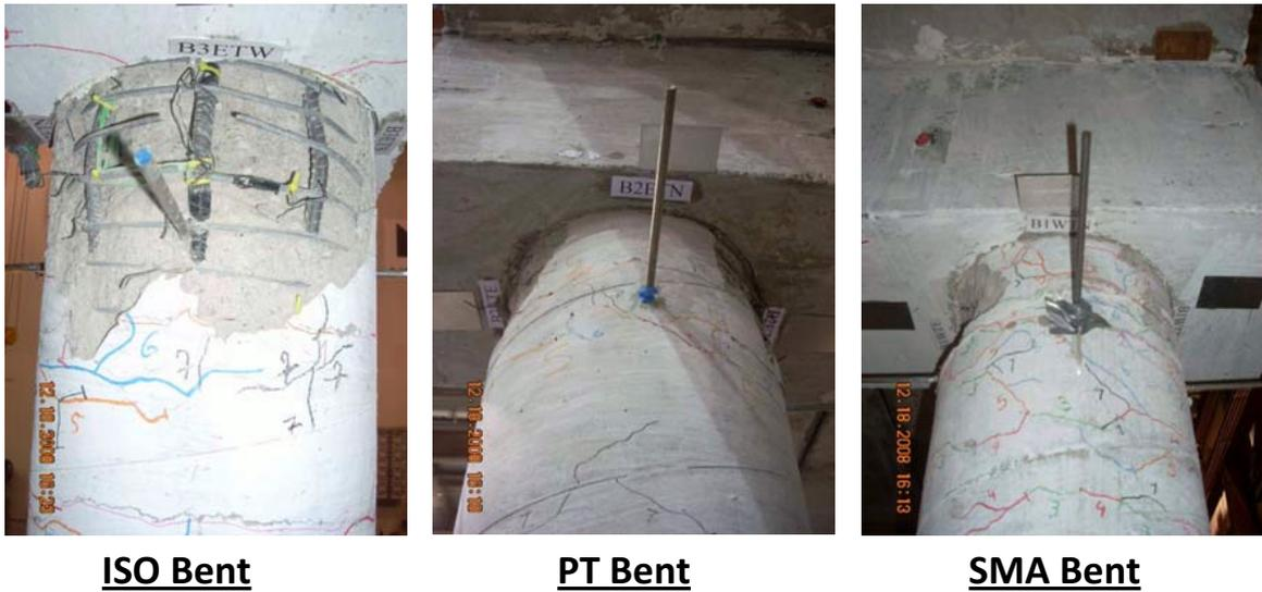
Figure 9. Top plastic hinge zones of ISO, PT and SMA bents after Run 7
