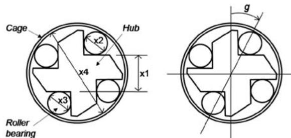
Figure 12. Fortini's clutch model illustration.
