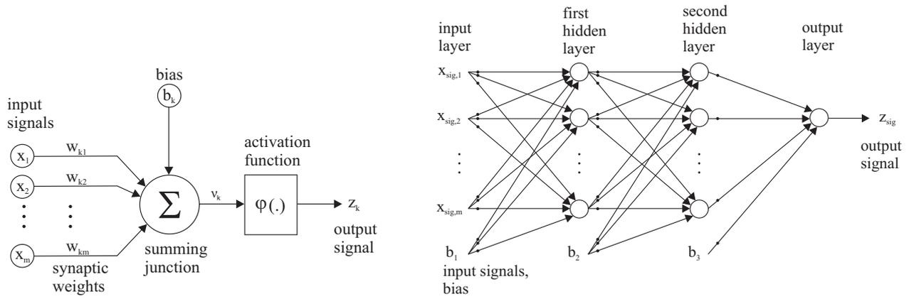
Figure 2. Constitution of a neural network; construct of a neuron (left) and feedforward neural network (right)
