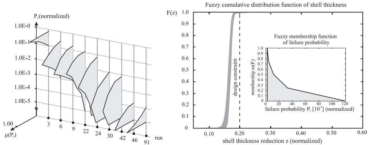
Figure 4. Fuzzy failure probabilities in selected optimization states (left) and (right) result of optimal design (run 91)
