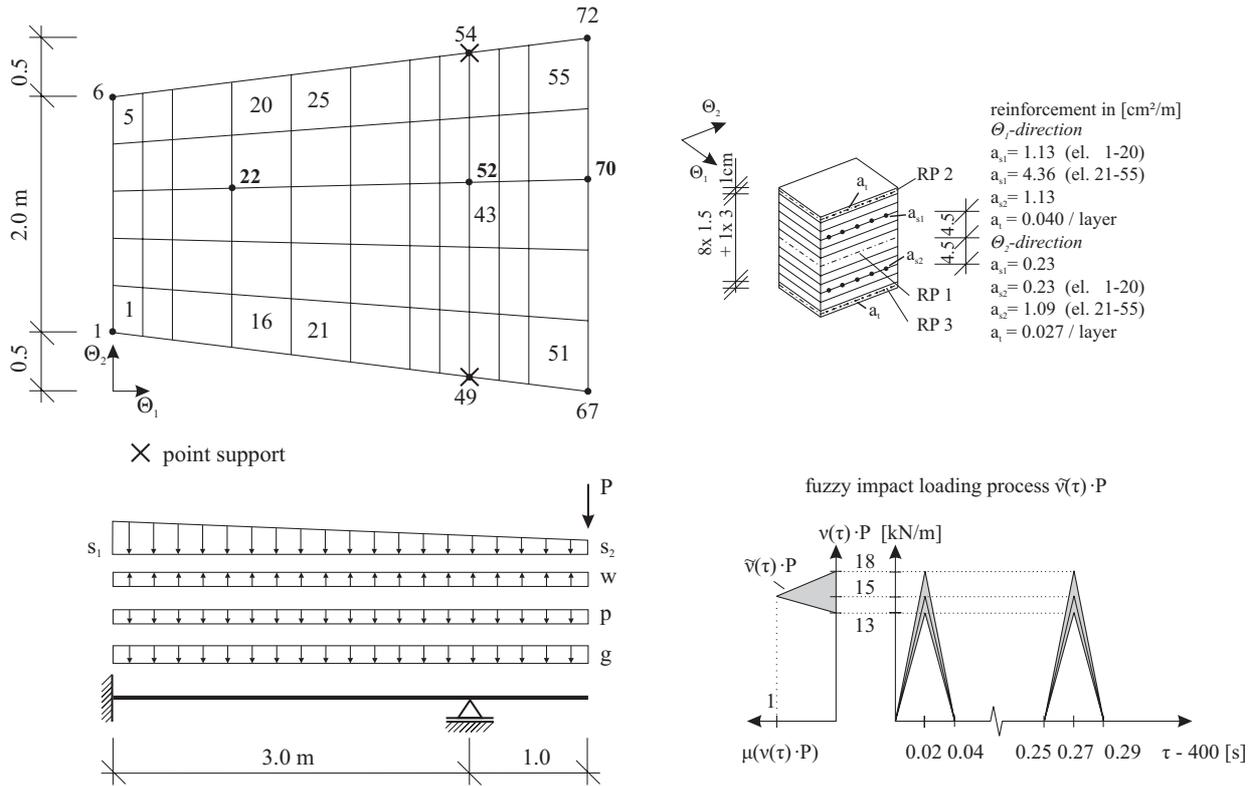
Figure 5. Geometry, FE model, and loading
