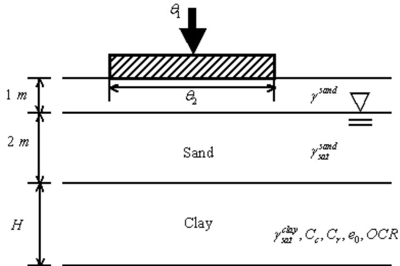
Figure 1 The cross section of the consolidation example.  $\theta_1$  and  $\theta_2$  are the bearing pressure and foundation width, respectively.
